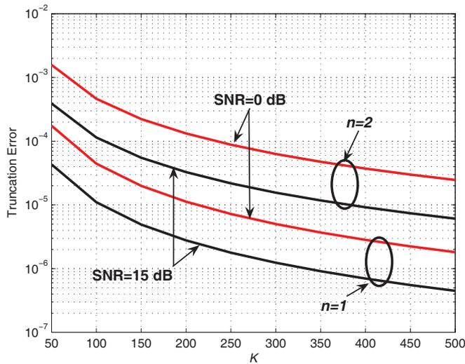
Fig. 3. The truncation error as a function of  $K$  ( $\sigma = 6$  dB).
