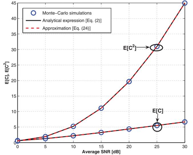
Fig. 1. The first and the second moments of the capacity ( $\sigma = 3$ ;  $K = 10$ ).
