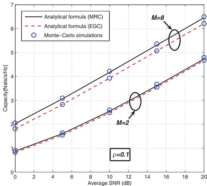
Fig. 4. Capacity of maximum ratio combining and equal gain combining in a correlated log-normal fading environment ( $\rho=0.1$ ) with  $M = 2$  antennas ( $\sigma_1 = 5$ ;  $\sigma_2 = 6$ ) and  $M = 8$  antennas ( $\sigma_1 = \dots = \sigma_4 = 5$ ;  $\sigma_5 = \dots = \sigma_8 = 6$ ).
