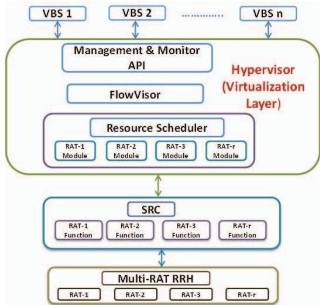
Fig. 1: LVN virtualization flow diagram.
