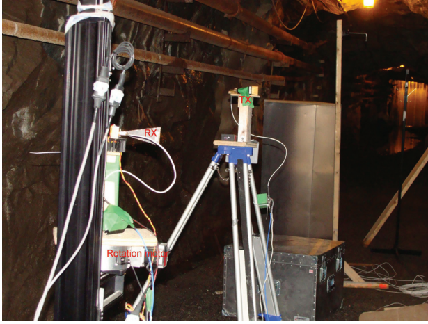
Fig. 7: Digital photograph for scattering measurement at 70 m mine gallery.
