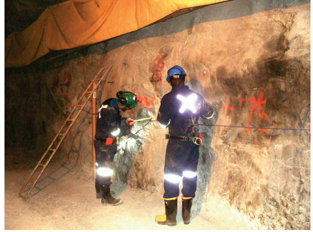
Fig. 2: Wall surface height measurement at 40 m mine gallery.
