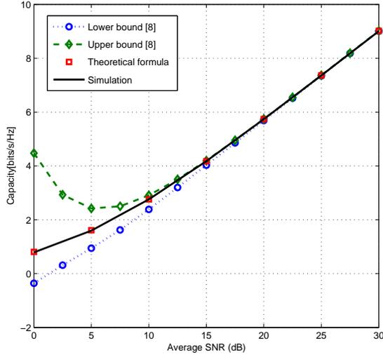
Figure 2: Capacity in log-normal fading ( $\sigma = 5$ ) for the SISO channel.
