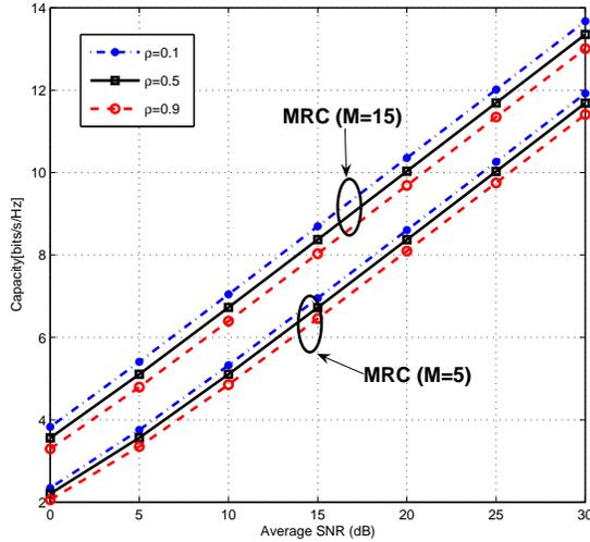
Figure 4: Capacity in log-normal fading ( $\sigma = 5$ ) of MRC for correlated branches.
