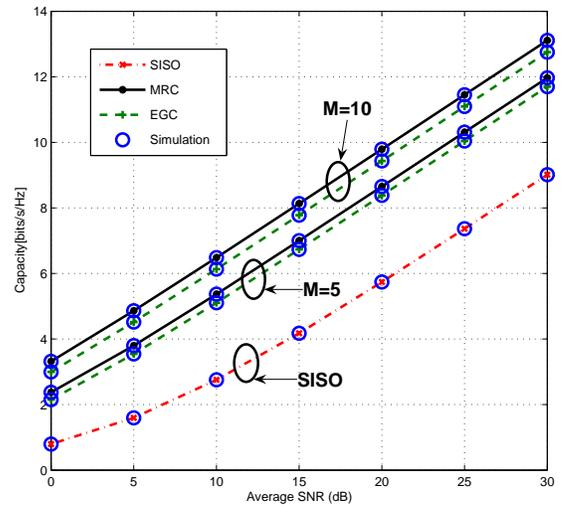
Figure 3: Capacity in log-normal fading ( $\sigma = 5$ ) for SISO, MRC and EGC ( $\rho = 0$  and  $K = 10$ ).
