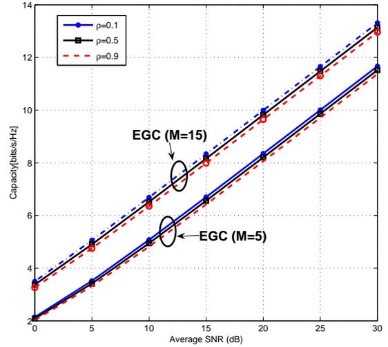
Figure 5: Capacity in log-normal fading ( $\sigma = 5$ ) of EGC for correlated branches.
