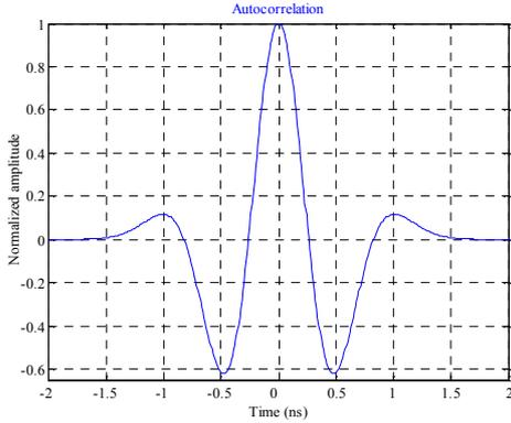
Figure 2. Autocorrelation of the 2<sup>nd</sup> order Gaussian pulse.
