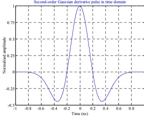
Figure 1. Second-order Gaussian derivative pulse shape.
