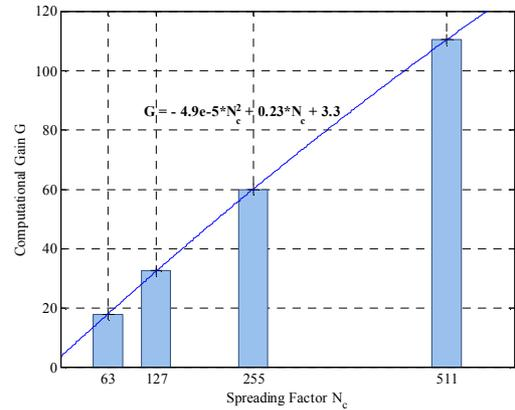
Figure 4. Gain in complexity with respect to the spreading factor for  $N_s=8$ .
