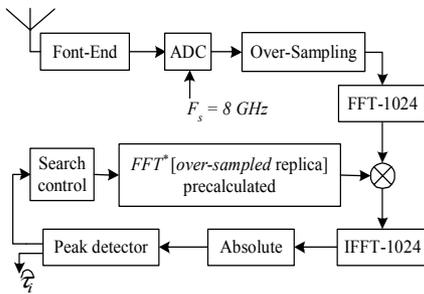
Figure 3. Block diagram of the proposed UWB fast acquisition scheme.
