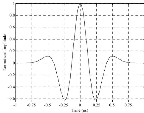
Figure 2. Autocorrelation of the 2<sup>nd</sup> order Gaussian pulse.
