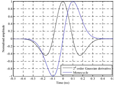
Figure 1. Gaussian Monocycle and Second-order Gaussian derivative waveforms in time domain.
