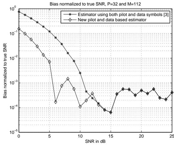
**Fig. 7.** Normalized bias of the estimators in the pilot-assisted case with number of iterations for the new estimator ( $I = 3$ ).
