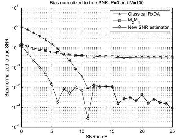
**Fig. 5.** Normalized bias of the estimators in the blind case with number of iterations for the new estimator ( $I = 10$ ).
