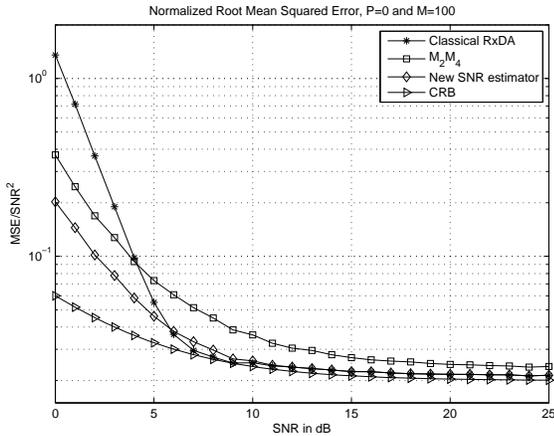
**Fig. 4.** True SNR normalized mean squared error of the estimators in the blind case with  $I = 10$ .
