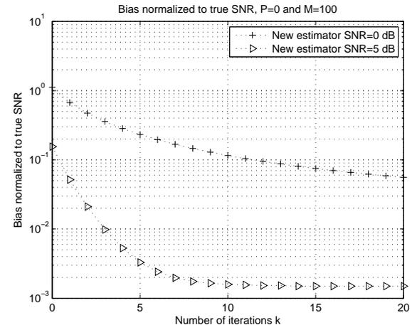
**Fig. 2.** Normalized bias of the new algorithm in the blind case.
