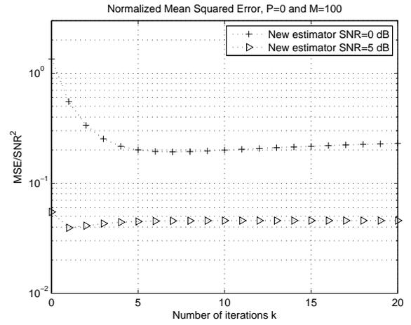
**Fig. 1.** True SNR normalized mean squared error of the new estimator in the blind case.
