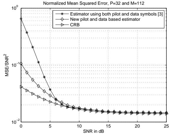
**Fig. 6.** True SNR normalized mean squared error of the estimators in the pilot-assisted case with number of iterations for the new estimator ( $I = 3$ ).
