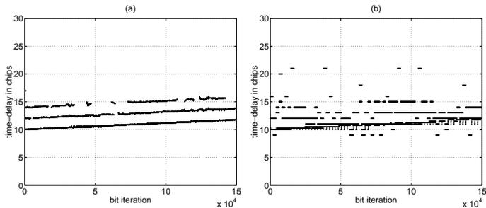
Fig. 4. Estimated time-delays  $\hat{\tau}_{p,n}$  for a (0, -6, -10) dB multipath power profile. (a): STAR. (b): 2D-RAKE.
