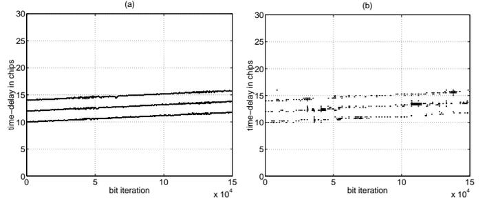
Fig. 2. Estimated time-delays  $\hat{\tau}_{p,n}$  for a (0, 0, 0) dB multipath power profile. (a): STAR. (b): 2D-RAKE.
