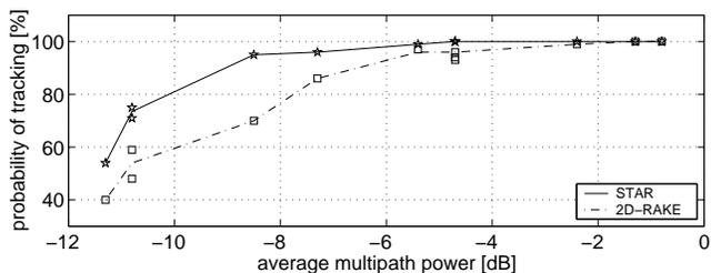
Fig. 6. Probability of tracking vs. the average multipath power for both STAR and the 2D-RAKE.
