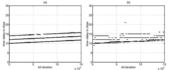
Fig. 3. Estimated time-delays  $\hat{\tau}_{p,n}$  for a (0, -3, -6) dB multipath power profile. (a): STAR. (b): 2D-RAKE.
