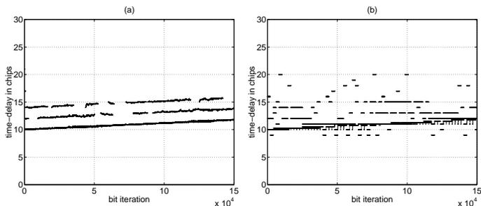
Fig. 5. Estimated time-delays  $\hat{\tau}_{p,n}$  for a (0, -10, -10) dB multipath power profile. (a): STAR. (b): 2D-RAKE.
