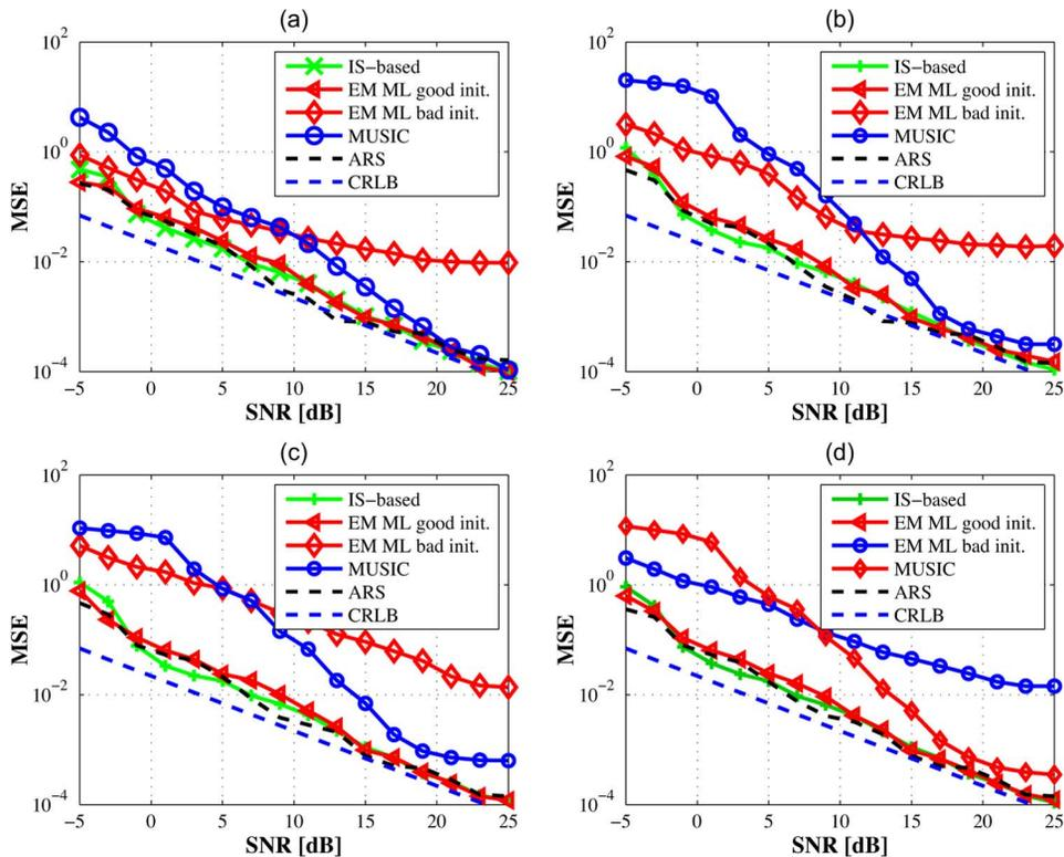
Fig. 6. Estimation performance of the IS-based, ARS-based, EM ML and the MUSIC-type algorithms vs. SNR in an active system for (a) 1st path, (b) 2nd path, (c) 3rd path, and (d) average over paths.
