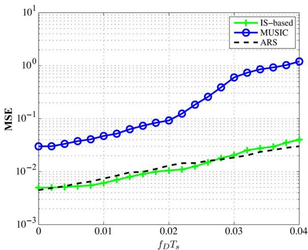
Fig. 10. Estimation performance of the IS-based, ARS-based and the MUSIC-type algorithms vs.  $f_D T_s$  at SNR = 10 dB in an active system.
