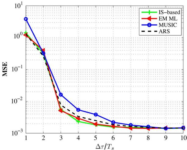
Fig. 8. Estimation performance of the IS-based, ARS-based, EM ML and the MUSIC-type algorithms vs.  $\Delta\tau$  in an active system.
