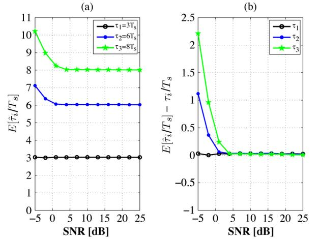
Fig. 5. Estimation bias of the IS-based algorithms vs. SNR (a)  $E\left\{\frac{\hat{\tau}_i}{T_s}\right\}$  and (b)  $E\left\{\frac{\hat{\tau}_i}{T_s}\right\} - \frac{\tau_i}{T_s}$ .
