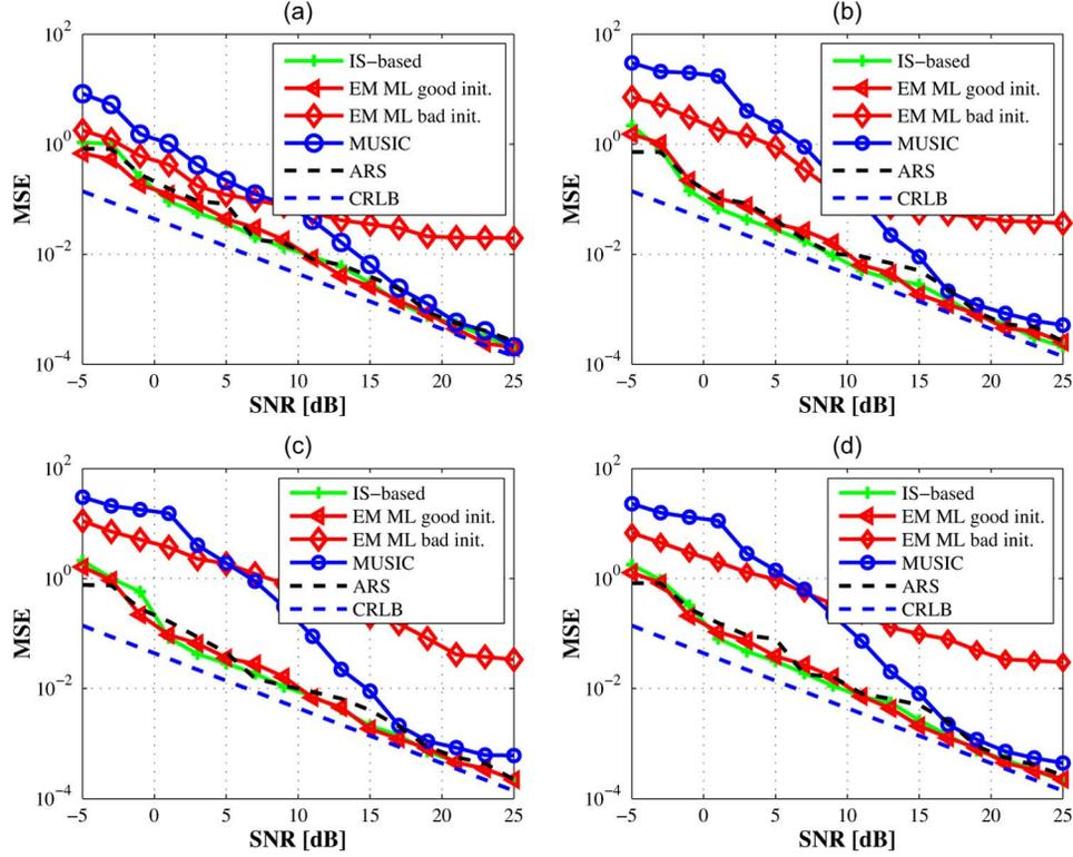
Fig. 7. Estimation performance of the IS-based, ARS-based, EM ML and the MUSIC-type algorithms vs. SNR in a passive system for (a) 1st path, (b) 2nd path, (c) 3rd path, and (d) average over paths.
