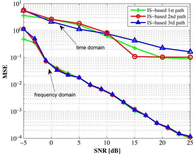
Fig. 3. Estimation performance of the IS-based algorithm in the time and frequency domains.
