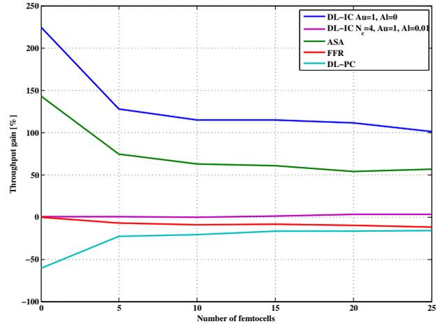
Fig. 4. Network throughput gains against a basic LTE HetNet without IC ( $\beta_m = 10^{-3}$ ).
