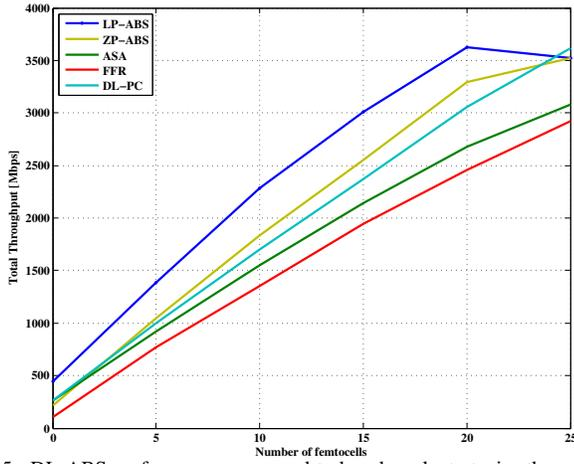
Fig. 5. DL-ABS performance compared to benchmark strategies through total network throughput.
