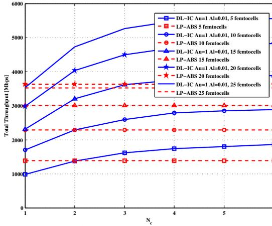
Fig. 6. DL-ABS performance compared to IC versus  $N_c$ .
