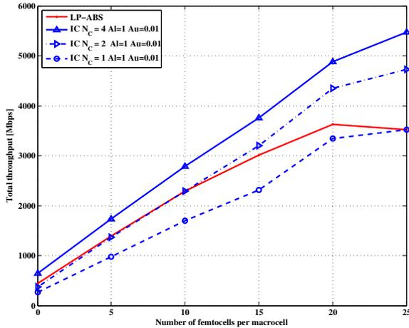
Fig. 7. DL-ABS performance compared to DL-IC versus the number of femtocells.
