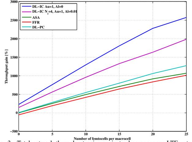
Fig. 3. Total network throughput gains against a homogeneous LTE network ( $\beta_m = 10^{-3}$ ).
