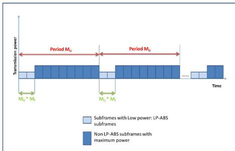
Fig. 1. LP-ABS subframes period and ratio illustration.
