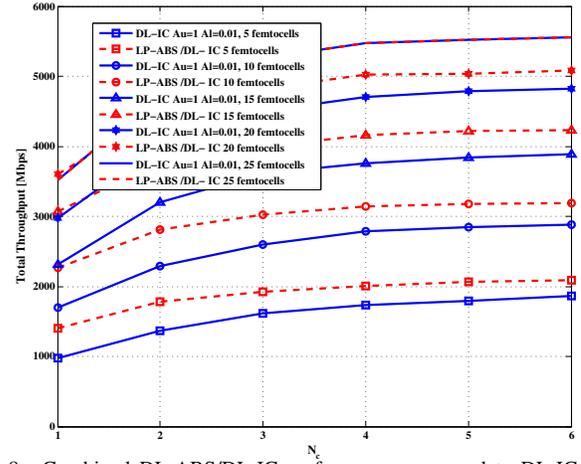
Fig. 8. Combined DL-ABS/DL-IC performance compared to DL-IC versus the number of constraints.
