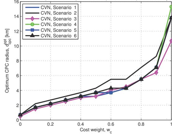
Fig. 4: Optimum CPC radius,  $d_{cpc}$  vs. cost weight,  $w_c$  for different scenarios ( table-I)
