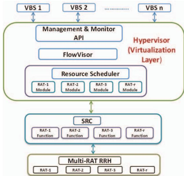
Fig. 1: LVN virtualization flow diagram.
