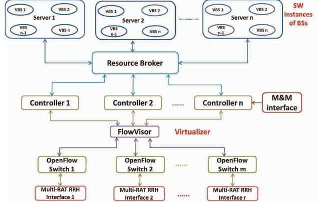
Fig. 2: CVN/RVN virtualization flow diagram.
