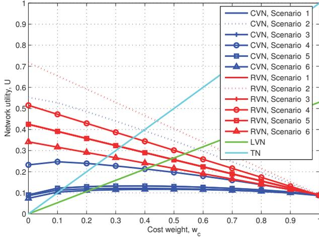
Fig. 5: Optimal network utility using optimal GP value,  $GP_{opt}$  vs. cost weight for different scenarios (Table-I)
