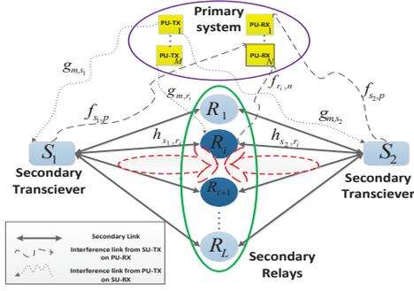
Fig. 1: Spectrum-Sharing System with Two-Way DF Relaying.
