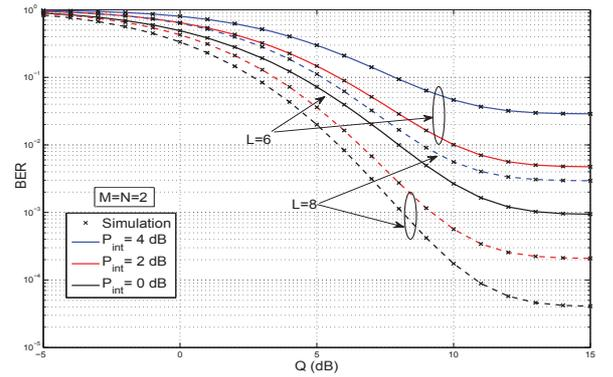
Fig. 3: BER vs.  $Q$  (dB) for  $L=6, 8$  and  $M = N = 2$ .
