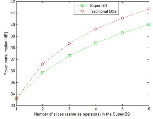
Fig. 3. Total power consumption vs #slices
