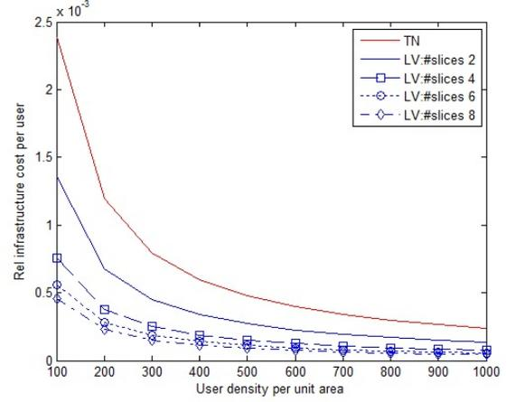
Fig. 2. Relative infrastructure cost vs user density (R=2 unit)
