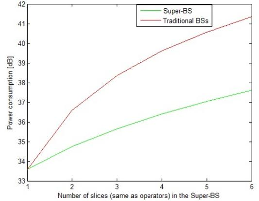
Fig. 4. Total power consumption vs #slices (shared antenna case)
