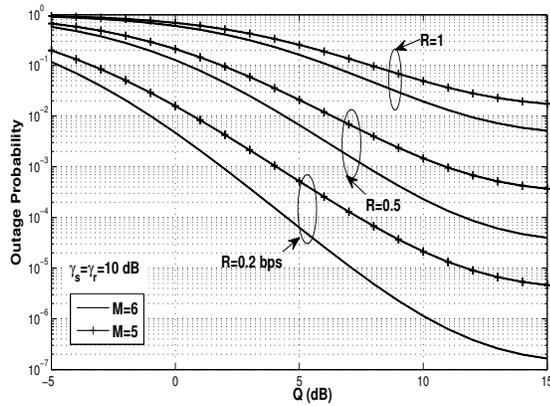
Fig. 3: Outage Probability vs.  $Q$ (dB) for different number of relays  $M=5,6$  for  $R_{min}=0.2, 0.5$  and  $1$  bits/s/Hz.
