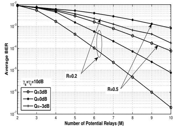
Fig. 5: Average BER vs. number of potential relays for  $Q = -3, 0, 3$  dB for both  $R_{min} = 0.2, 0.5$  bits/s/Hz.
