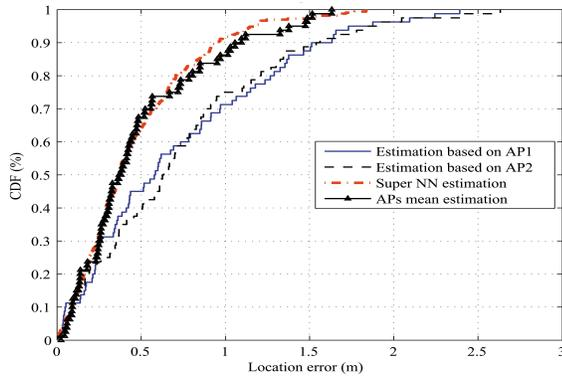
Fig. 8. CDF plots of the position estimation errors for the testing data at a receivers' separation distance  $D = 80$  m using several localization techniques.
