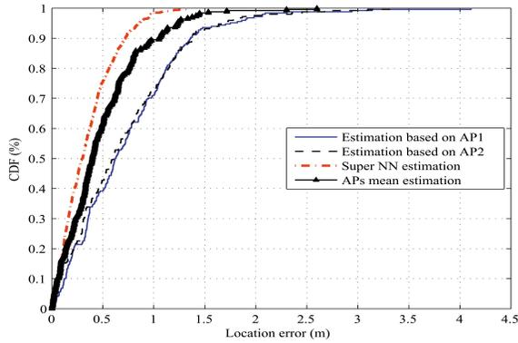
Fig. 7. CDF plots of the position estimation errors for the training data at a receivers' separation distance  $D = 80$  m using several localization techniques.
