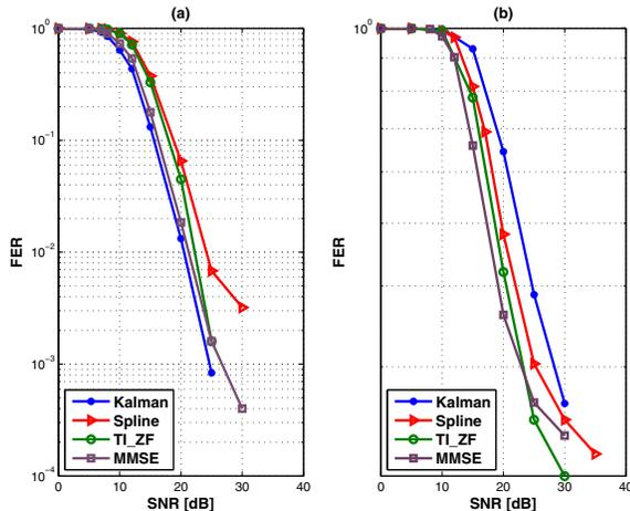
Fig. 3. FER vs. SNR for the estimation schemes over (a) slow fading channel and (b) fast fading channel.
