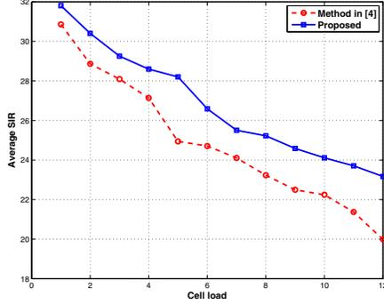
Fig. 8. Average SIR for different cell loads.
