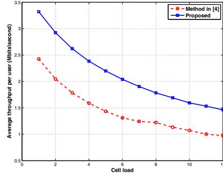
Fig. 9. Average throughput per user for a switched-beam OFDM system.
