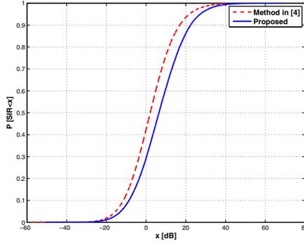
Fig. 7. CDF of the SIR for a cell load of 12 users.
