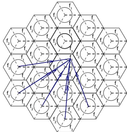
Fig. 1. Frequency reuse pattern for multi-cell OFDM systems.
