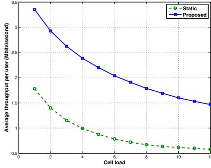
Fig. 6. Average throughput per user for static and dynamic subcarrier allocation strategies.
