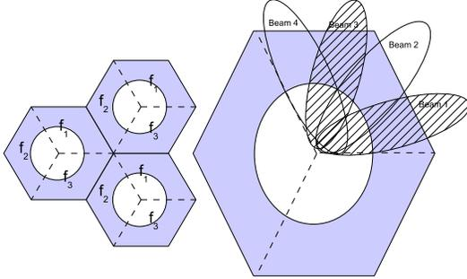
Fig. 2. Frequency assignment for a multi-cell switched-beam OFDM system.
