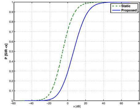
Fig. 4. CDF of the SIR for a cell load of 12 users.
