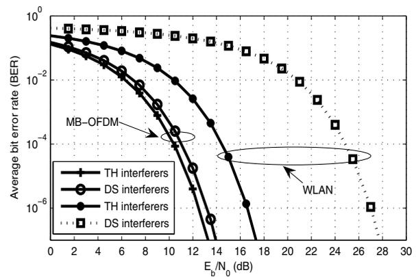
Fig. 4. Comparison of the BER performance between 802.11a OFDM and MB-OFDM in the presence of  $N_u = 20$  interferers
