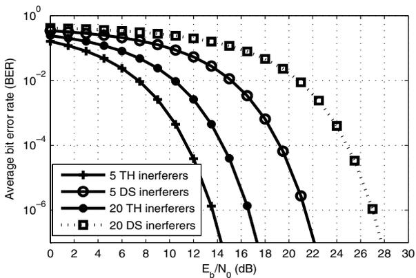
Fig. 3. Average BER versus  $E_b/N_0$  of the WLAN 802.11a system in the presence of TH and DS UWB interference
