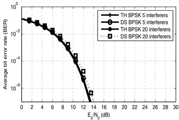
Fig. 2. Average BER versus  $E_b/N_0$  of the MB-OFDM system in the presence of TH and DS UWB interference
