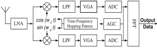
Fig. 1. Receiver architecture for a MB-OFDM system
