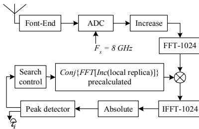
Figure 3. Block diagram of the proposed UWB fast acquisition system.
