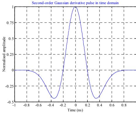
Figure 1. Second-order Gaussian derivative pulse shape.
