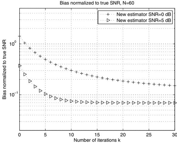
Fig. 3. Normalized bias of the new algorithm with QPSK signals,  $N = 60$ .
