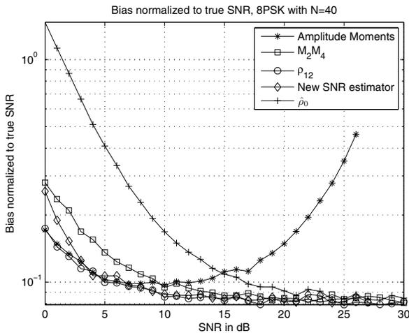
Fig. 8. Normalized bias of the estimators with 8-PSK signals,  $N = 40$  and  $I = 20$ .
