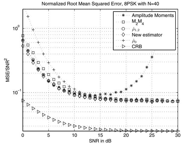
Fig. 6. True SNR normalized mean squared error of the estimators with 8-PSK signals,  $N = 40$  and  $I = 20$ .
