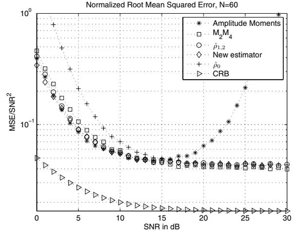
Fig. 5. True SNR normalized mean squared error of the estimators with QPSK signals,  $N = 60$  and  $I = 20$ .
