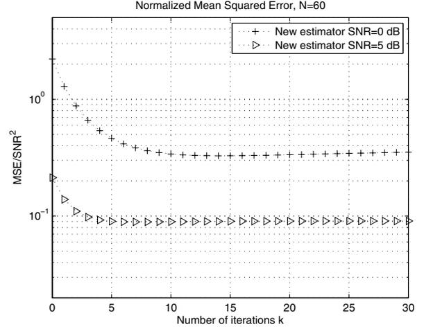
Fig. 2. True SNR normalized mean squared error of the new estimator with QPSK signals,  $N = 60$ .
