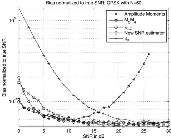
Fig. 7. Normalized bias of the estimators with QPSK signals,  $N = 60$  and  $I = 20$ .
