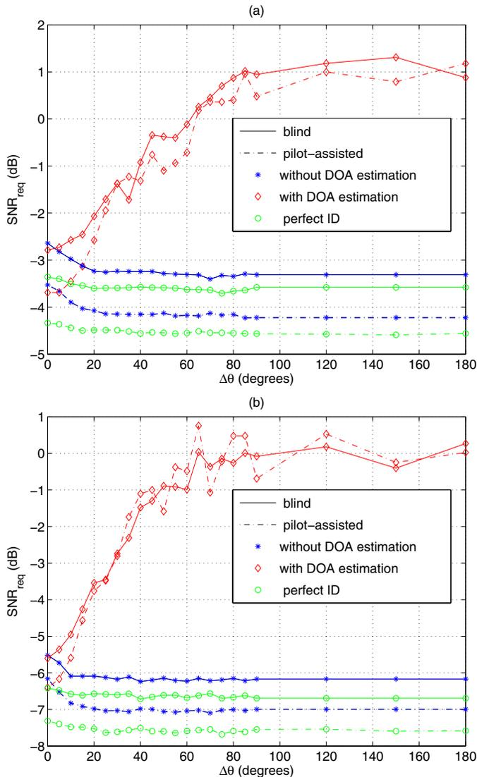
Fig. 1. Link-level simulation results of array receiver STAR at 5 Km/h with and without DOA estimation, both in the pilot-assisted and blind modes, in terms of required SNR at a target BER of 1% versus the angular spread  $\Delta\theta$ , using (a):  $M = 8$  and (b):  $M = 16$  ULA antenna elements.
