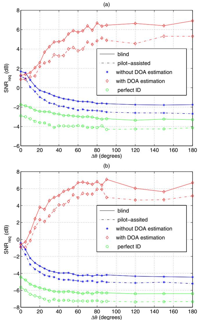
Fig. 2. Link-level simulation results of array receiver STAR at 50 Km/h with and without DOA estimation, both in the pilot-assisted and blind modes, in terms of required SNR at a target BER of 1% versus the angular spread  $\Delta\theta$ , using (a):  $M = 8$  and (b):  $M = 16$  ULA antenna elements.
