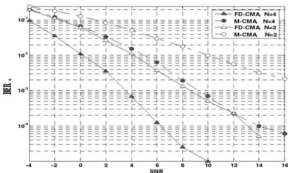
Figure 5. BER performance versus SNR in Type -B Channels when the number of elements is varied.
