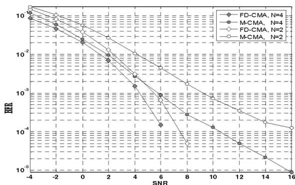
Figure 4. BER performance versus SNR in Type -A Channels when the number of elements is varied.
