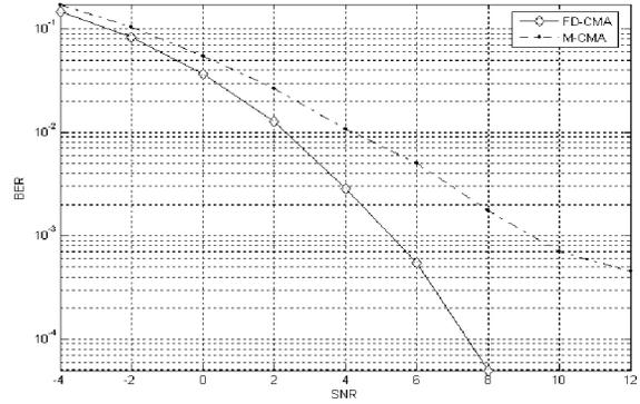
Figure 2. BER performance versus SNR in Type -A Channels for  $\tau_2=0.2 T_s$  and  $\tau_3=0.8 T_s$ .
