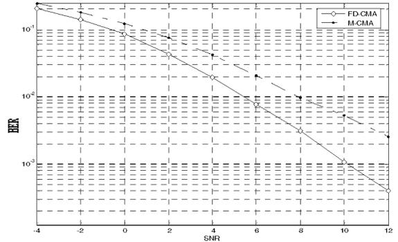
Figure 3. BER performance versus SNR in Type -B Channels for  $\tau_2=0.2 T_s$  and  $\tau_3=0.8 T_s$ .
