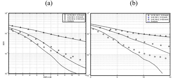
Fig. 1. Analytical and simulated BER vs. SNR in dB for (a): MT-CDMA,  $L = 64$ ,  $N_c = 3$ , DBPSK and (b): MC-DS-CDMA  $L = 32$ ,  $N_c = 3$ , DBPSK.
