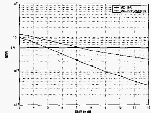
Fig. 3. BER vs. SNR in dB of MT-CDMA MC-ISR,  $L = 64$ ,  $N_c = 3$ ,  $U = 8$ , with and without full interference suppression (i.e., with and without ICI suppression).
