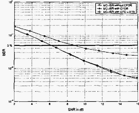
Fig. 1. BER vs. SNR for MT-CDMA MC-ISR,  $L = 96$ ,  $N_c = 7$ ,  $U = 5$ , with and without CFOR.
