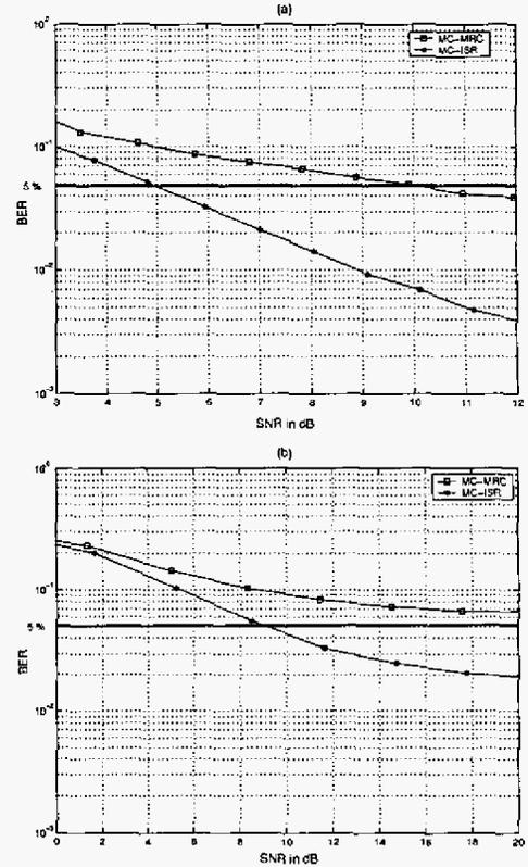
Fig. 2. BER vs. SNR in dB of MC-MRC and MC-ISR with (a): MT-CDMA,  $L = 64$ ,  $N_c = 3$ ,  $U = 8$ , DBPSK and (b): MC-DS-CDMA,  $L = 32$ ,  $N_c = 3$ ,  $U = 8$ , DBPSK.
