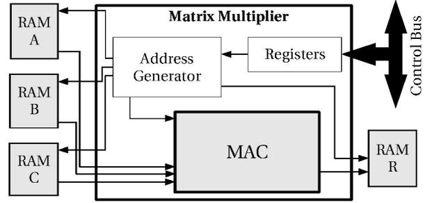
**Figure 3.** Matrix Multiplier architecture.
