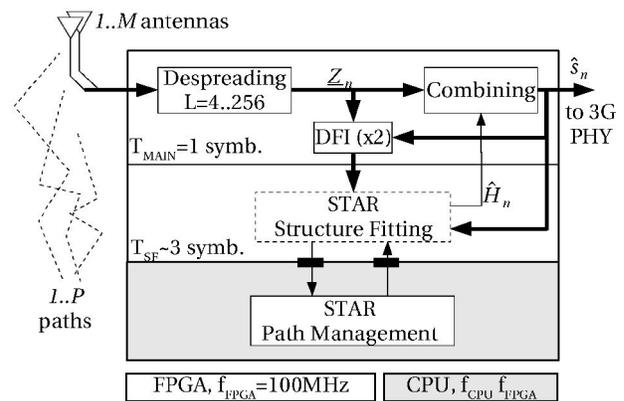
**Figure 1.** Global architecture of the PHY layer in a STAR-enabled 3G base station receiver. Black boxes represent distributed RAM.
