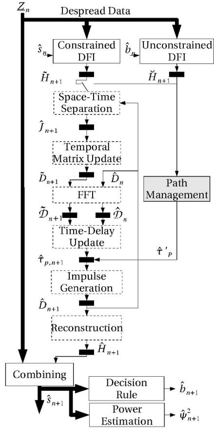
**Figure 2.** Pipeline structure of STAR. In FPGA: white solid-line blocks form the main data path ( $T_{\text{MAIN}}=1$  symbol), white dotted-line blocks make up the structure-fitting pipeline ( $T_{\text{SF}}\sim 3$  symbols). In CPU: the gray block performs adaptive path management ( $T_{\text{CPU}}\sim 100$  symbols). Black boxes are dual-port RAM elements.
