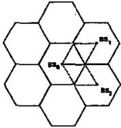
Fig. 1. The hexagonal cell geometry with first layer of surrounding cells.
