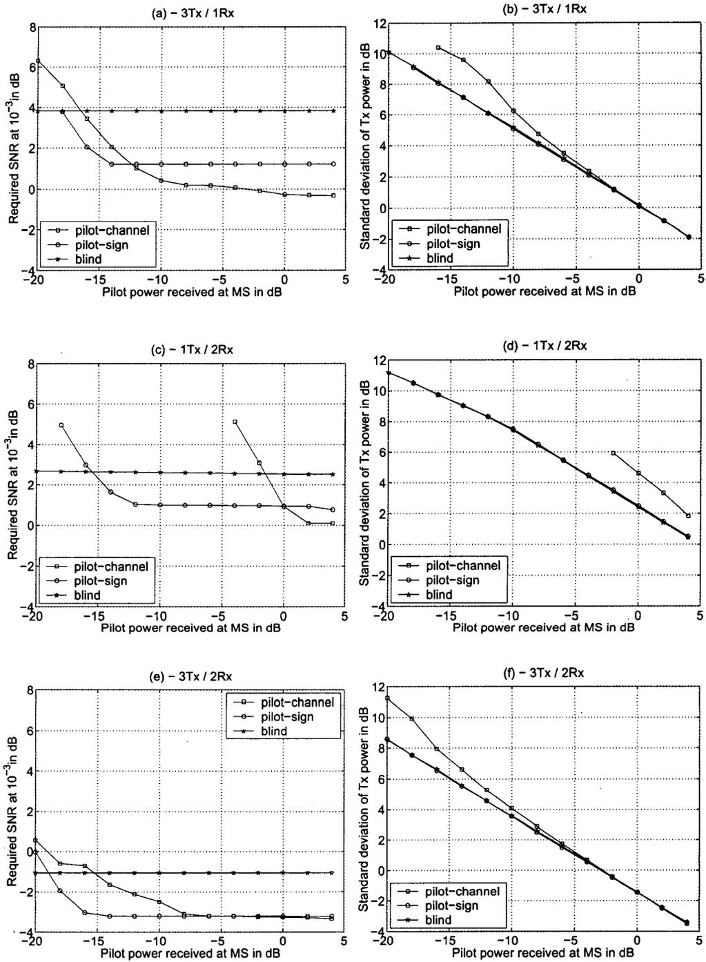
Figure 1: Downlink results in the three selected (Tx/Rx) antenna configurations - (a),(c),(e): Required SNR at a BER of  $10^{-3}$  after FEC decoding, and (b),(d),(f): the corresponding standard deviation of the data transmitted power, both versus the average received pilot power, for the three STAR versions.
