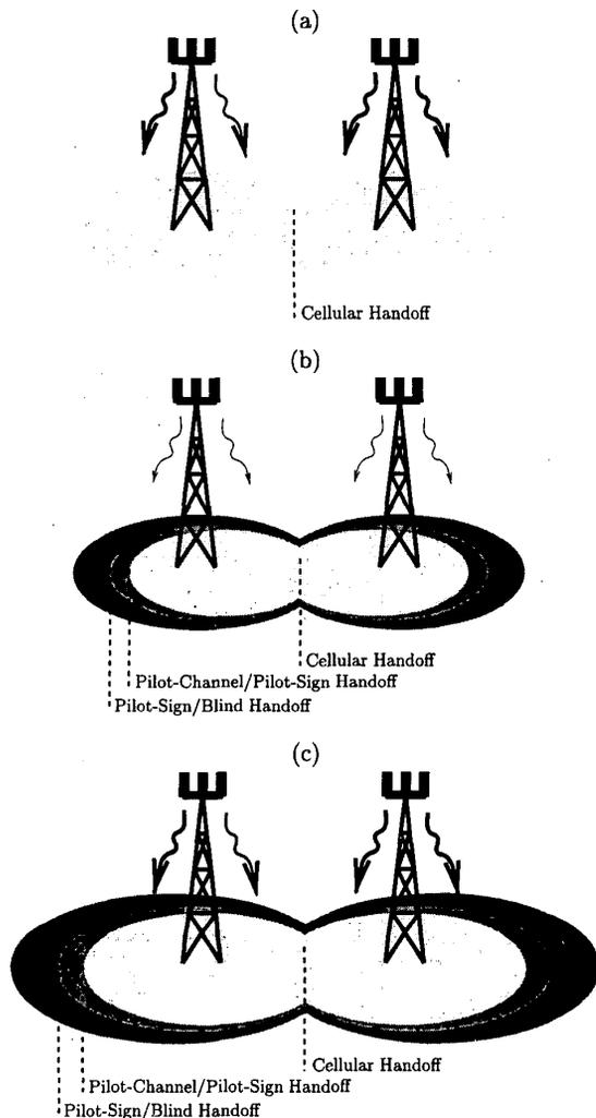
Figure 2: Benefits of modulation&identification "handoff" between STAR versions. (a) to (b): Increased capacity with reduced pilot-power transmission. (a) to (c): Increased coverage and reduced call drops.
